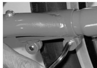
Fig 3: Tighten sideloader sleeve
