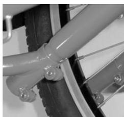
Fig 1: Sideloader sleeves
